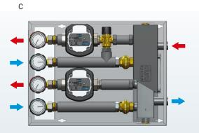
In case of a lateral position, it is recommended that on the top of the coupling manifold system or the manifold an automatic air-vent should be installed and at the bottom of the coupling manifold system or the manifold a drain valve should be installed.
