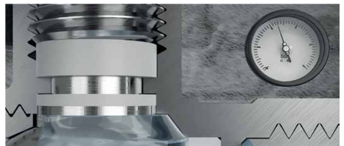
Pressure increase - seal compression
