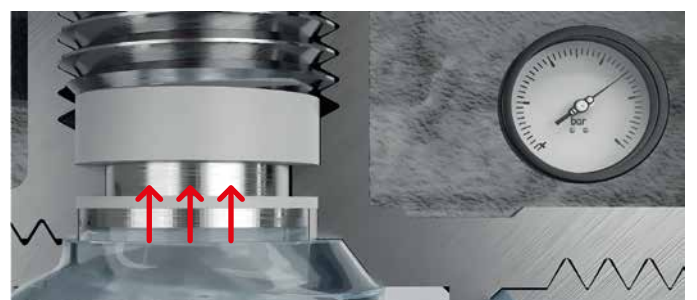
Pressure increase - seal compression
